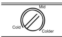
Place it in a central position to set an optimal temperature for normal use. The more you turn the knob clockwise, the lower the temperature in the appliance will be. The more you turn the knob counterclockwise, the higher the temperature in the appliance will be. Make sure the desired temperature has been reached by using a thermometer.
