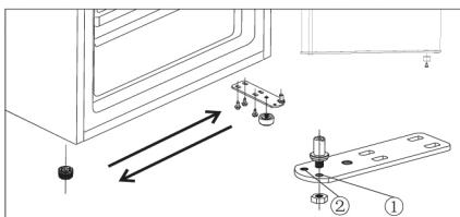
Screw down the door hinge and the feet back on the other side.
