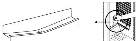
Make sure that the drain gully and the drain opening are not blocked so that the water produced in the refrigerator can always flow off unobstructed.
