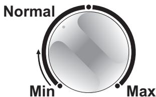
Place it in a central position to set an optimal temperature for normal use. The more you turn the knob clockwise, the lower the temperature in the appliance will be. The more you turn the knob counterclockwise, the higher the temperature in the appliance will be. Make sure the desired temperature has been reached by using a thermometer.
